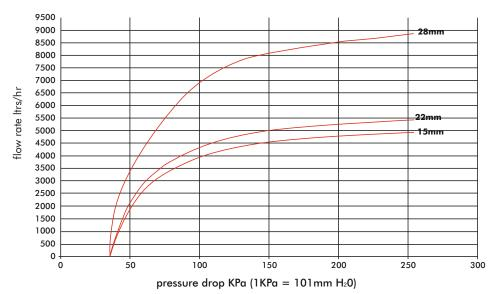
these values are obtained with: Inlet pressure 8 bar and outlet pressure 3 bar
